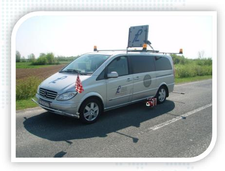
Zehntner ZDR 6020 (mounted on vehicle) is used for dynamic measuring of night visibility (retroreflection) of road markings (horizontal signalization). The ZDR 6020 is a dynamic measuring system for the fast and precise recording of the night visibility and important ambient data of long distances or large areas.
