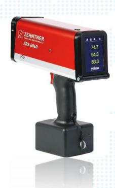
• Zehntner ZRS 6060 is device used for measuring retroreflection of traffic signs (vertical signalization). Zehntner ZRS 6060 uses LED lighting and a 3.5 " high-resolution color touch screen with adjustable angle. Device is used for all types and colors of retroreflective material and automatically detects the color of retroreflective material. Device stores GPS coordinates and measurements can be evaluated with the included mapping and data analysis software "MappingTools".
