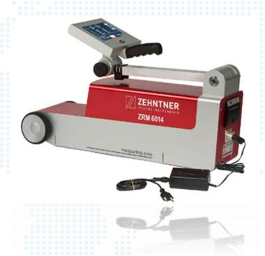
Zehntner ZRM 6013 and ZRM 6014 are used for the measuring day and night visibility of road markings (horizontal signalization).
